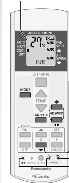
Press and hold for approximately 10 seconds to show temperature setting in °C or °F.
